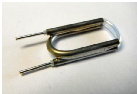
Fig. 2 Turn VHF Coaxial Transformer
